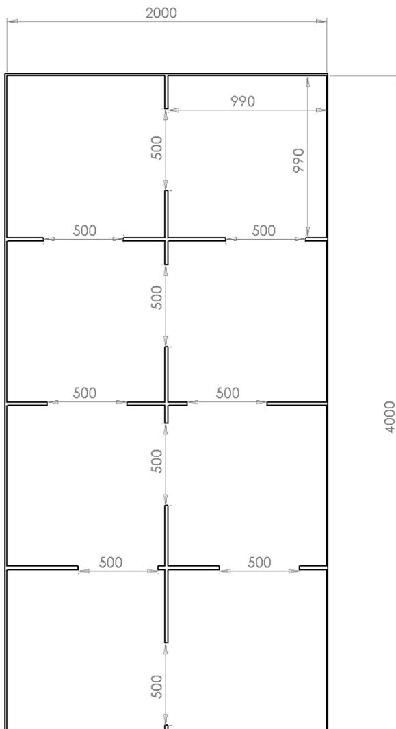
The competition table is 4000 mm x 2000 mm with a 100 mm exterior wall. The table will be split into eight 990 mm x 990 mm rooms with an internal wall height of 100 mm. Each room will have a 500 mm wide entrance and exit. The positioning of the entrance and exit to each room will be different.
